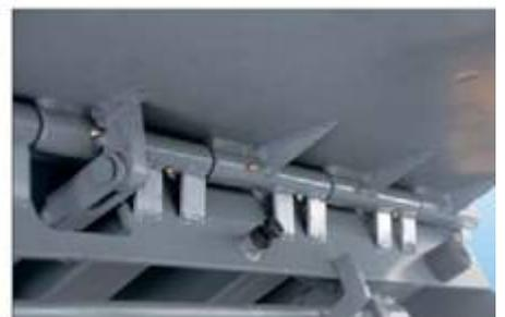
Fully hydraulic dock levelers offer Button-operation to control deck and lip functions, including deck raise and lip kick out and return to stored position. And lip bumper and grease fitting on lip hinge are standard with each unit.
